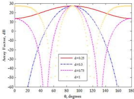
**Figure 5.** The normalized array factor of the binomial array of  $N = 11$  sources, with spacing between elements varying from  $0.25\lambda$  to  $\lambda$ . The binomial array with spacing between elements less than or equal to  $\lambda/2$  does not have secondary lobes.
