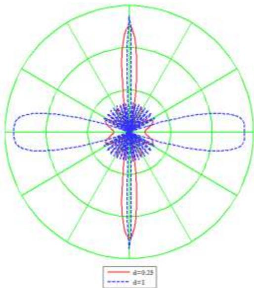
**Figure 8. The radiation patterns of the Dolph-Chebyshev array for  $N = 11$  with various spacings:  $d = 0.25\lambda$  and  $d = \lambda$ .**
