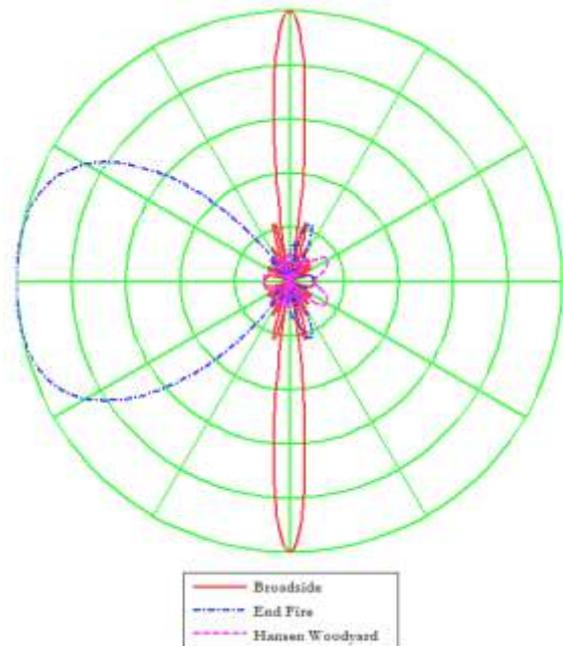
**Figure 4. Radiation patterns of Broadside, End-Fire and Hansen-Woodyard arrays for  $N = 11$  and  $d = 0.25\lambda$ . For a rather large uniform array, the Hansen-Woodyard array can also improve directivity for spacing between the elements approximately equal to  $\lambda/4$ .**
