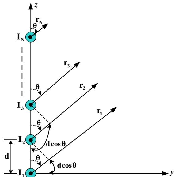
Figure 2. Geometry of the problem, showing a linear antenna array of  $N$  sources.
