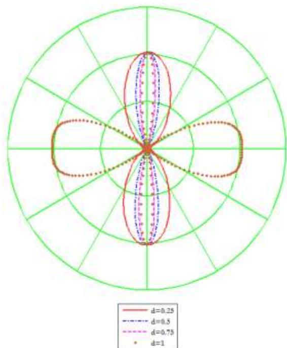
**Figure 6.** Radiation patterns of the binomial array of  $N = 11$  sources, with spacing between elements varying from  $0.25\lambda$  to  $\lambda$ . The binomial array usually has the smallest secondary lobes.
