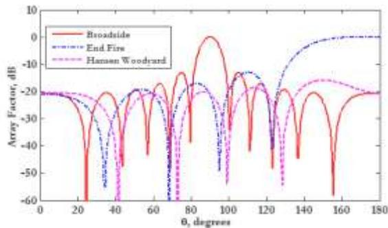
**Figure 3. Normalized array factor of Broadside, End-Fire and Hansen-Woodyard arrays for  $N = 11$  and  $d = 0.25\lambda$ . The curve for the array factor of Hansen-Woodyard shows that the first desired maximum depends on the progressive phase  $\beta$ . If  $\beta = \mp kd$ , the first desired maximum tends either towards  $0^\circ$  ( $\beta = -kd$ ), or towards  $180^\circ$  ( $\beta = kd$ ).**
